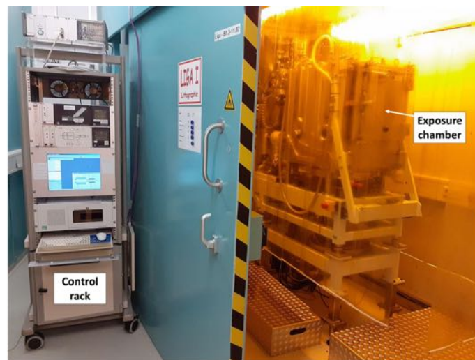
Figure 5.2.: Picture of the LIGA I beamline [51]. Sample and mask inside the exposure chamber on the right, control rack to set irradiation values on the left.
