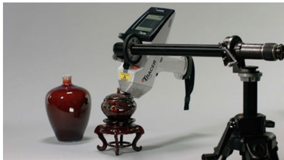
Fig. 7.43 A handheld XRF device mounted for analysis of art pieces. Permission granted by Bruker Nano GmbH
