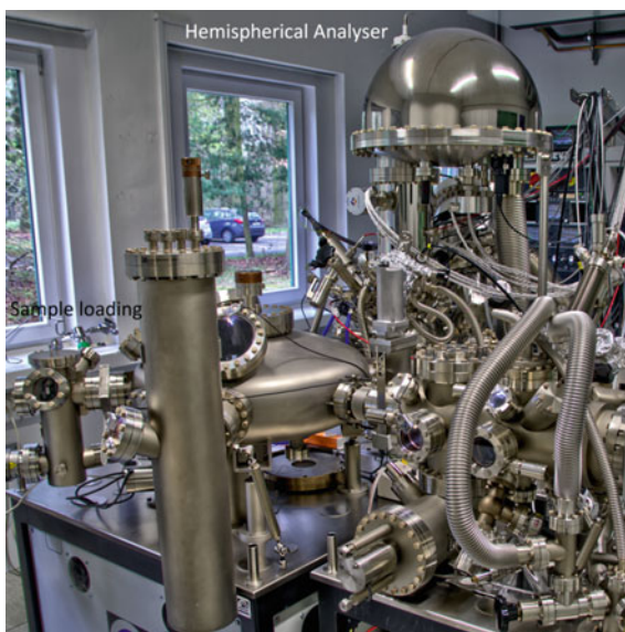
Fig. 7.11 Technical implementation of XPS with the typical hemispherical electron energy analyser attached to a larger system with sample loading and other techniques. Copyright Forschungszentrum Jülich/Tobias Wegener
