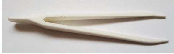
Fig. 2.55 Tweezers, a simple yet efficient way of increasing distance to radioactive material
