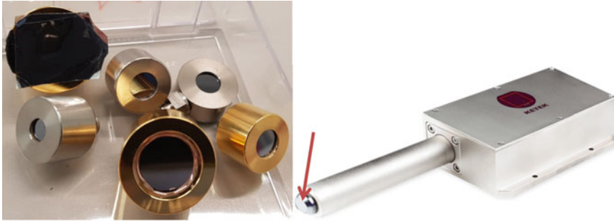
Fig. 2.42 Left: Different sizes of commercial depleted silicon detectors for charged particle detection. The central window represents the sensitive silicon crystal of here 25, 50, or 150 mm 2 . All but one detector feature a backside connector. The top-left is covered by a foil making it more dE/dx sensitive but reducing its resolution. Own work. Right: a silicon-drift-detector (arrow) for X-rays integrated with electronics into a compact package. Courtesy of KETEK GmbH
