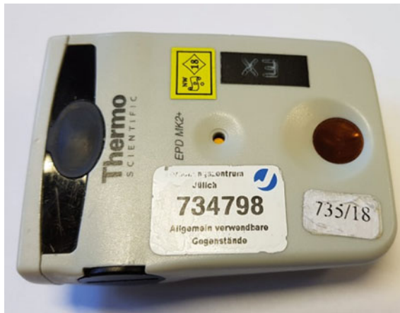
Fig. 2.58 An EPD used for direct personal dose rate estimation of photon ( \gamma ) and electron ( \beta ) doses. Correct placement for catching, technical properties and orientation towards the radiation source represent the main difficulties in application
