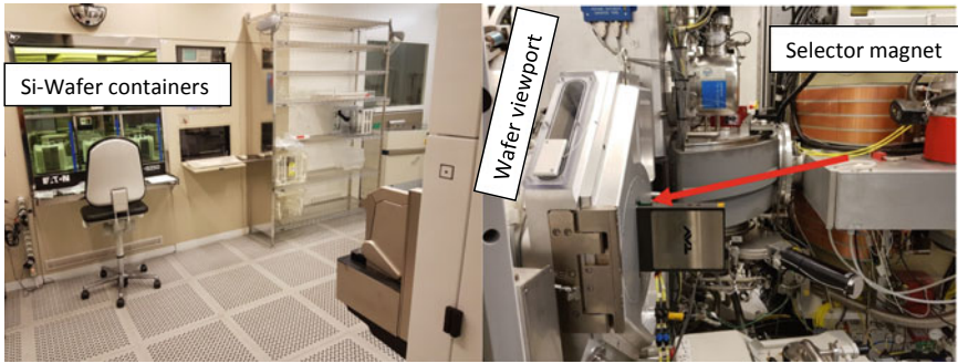
Fig. 5.12 A 70 kV implanter with attached clean room for 300 mm wafer doping (left). In the clean room the operator attaches wafer boxes to the automatic manipulator of the implanter (right). Its ion source produces a multitude of species from gases and vapours. A magnet selects the ion species and directs the beam (arrow) onto the wafer. Copyright Forschungszentrum Jülich/Sören Möller
