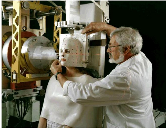
Figure 4. Treatment positioning at LBL facility: The patient was fixed in front of the beam exit window at the left side. Also, the compensator, consisting of many individual PMMA rods is visible (Source: imaging archive of the Lawrence Berkeley National Laboratory, © 2010–2019 The Regents of the University of California, Lawrence Berkeley National Laboratory).
