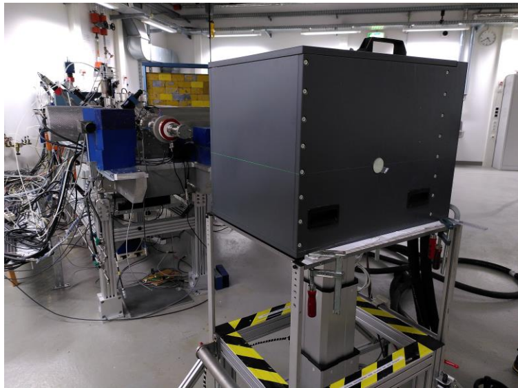
PTB's primary standard of the unit Gy in UHPDR reference electron beam
