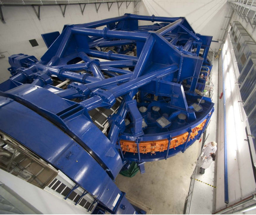
Fig. 3. The HIT 360° ion beam gantry.
