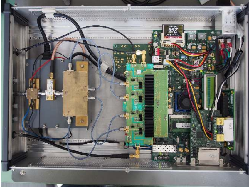
Figure 5.4: The Photo of KAPTURE is showing the 1-4 splitter, the V connection cables to the four sampling channels (consisting of a T/H unit and 500 MHz ADC each) on the digitizing board, the FPGA board below, and the PCI-Express connector (bottom right) for the connection to the control PC. Courtesy of Michelle Caselle.
